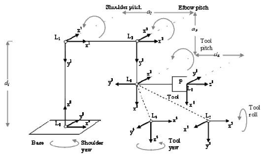
Figure 1: Link coordinate diagram for the SVR with horizontal tool
