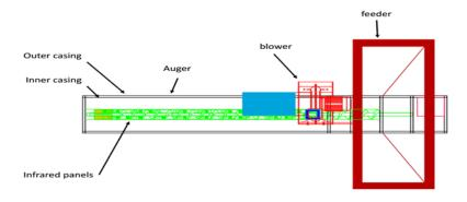
Figure 1: Top view of the gelatinizer
