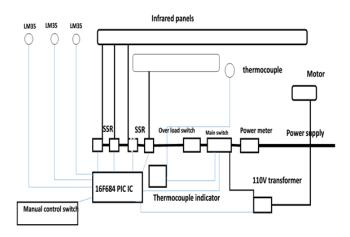
Figure 5: Diagram of the main controlling system
