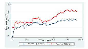
Figure 6: Rice flour temperature variation at the flour input and output of the FIR gelatinizer
