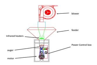
Figure 2: Front view of the gelatinizer
