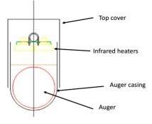
Figure 4: Arrangement of the FIR heaters
