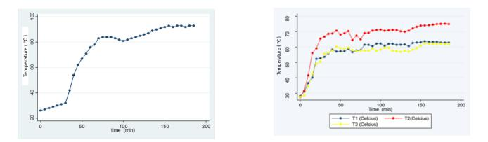
Figure 7 (a): Machine inner surface temperature variation Figure 7 (b): Machine outer surface temperature variations
