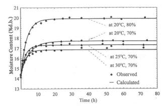
Figure 3: Water adsorption characteristics of polished rice under fluidizing conditions
