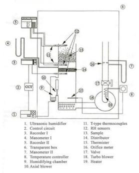
Figure 1: The experimental apparatus
