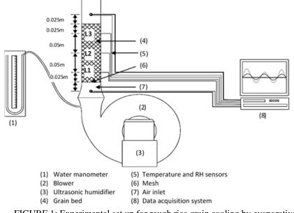
FIGURE 1: Experimental set up for rough rice grain cooling by evaporative cooling.
