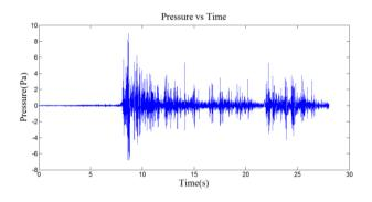
Figure 2. The pressure variation of the thunder obtained from the sensitivity of the conditioning amplifier100 mV/Pa  $\,$
