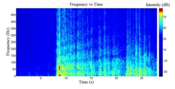
Figure 3. The frequency variation of the recorded thunder signal represents with time. All the frequency components less than 500 Hz are analyzed in this study by the relative power and the dominant frequencies are obtained from the maximum power dissipation.
