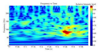
Figure 5. The frequency variation of the recorded peal obtained from the spectrogram generated by S-transformation
