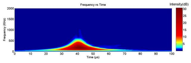
Figure 3. S-Transform spectrum of a positive narrow bipolar pulse.
