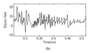
Figure 3. A semi-regular pulse burst of microsecond scale pulse associated with a chaotic leader; (a) fast electric field signature; (b) expanded time scale.
