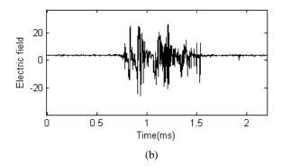
Figure 1. A semi-regular pulse burst of microsecond scale pulse associated with a K-change in ground flash; (a) slow electric field signature; (b) Fast electric field.
