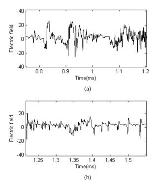
Figure 2. The Same pulse burst in Fig. 1, but displayed on an expanded time scale (a) beginning of pulse train with an irregular pulse; (b) the last portion of pulse train with regular pulses.
