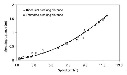
Figure 6: Variation of theoretical and observed breaking distance with velocity. Continuous line: The polynomial fit for the theoretical values. The dotted line: The polynomial fit for the theoretical values.
