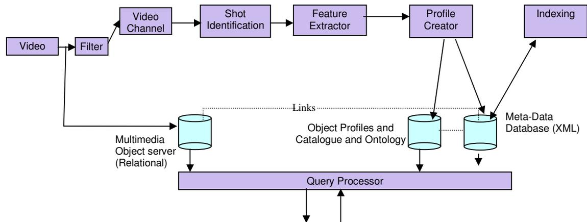
**Figure 3.1: System architecture**
